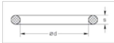
Dimensional drawing for the spare O-ring gaskets for ISO-KF flange connections
