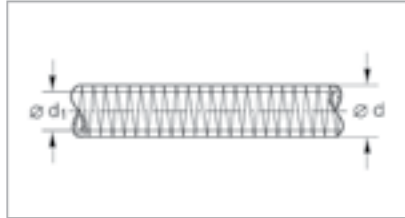
Dimensional drawing for the PVC vacuum hoses
