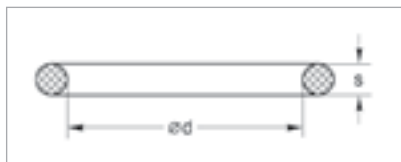
Dimensional drawing for the spare O-ring gaskets for ISO-KF flange connections
